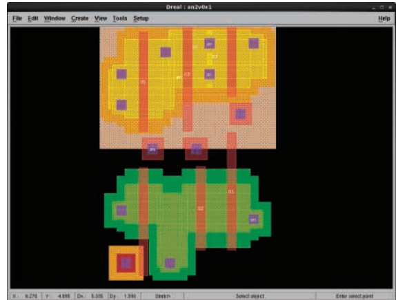
Fig.11 The layout in case of no complement poly layer
