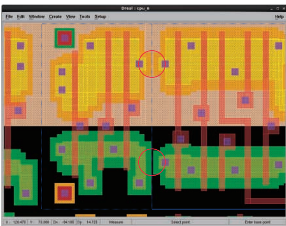
Fig.16 The example minimum distance fault between cells. Blue line is cell border. Red line is area there is fault.
