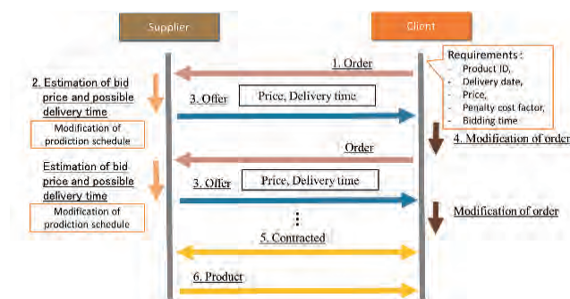
Fig.4 Negotiation flow between a client and a supplier
